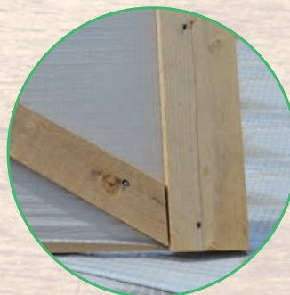
Detail corrosion interlaced paper
